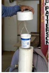
The first BP charges to be tested were like my normal charges..we used igniterman igniters (to save our ematches) They had two layers of medical glove finger tips, instead on the normal one. They were then wrapped with tape in an attempt to contain is a bit longer. There was no shrapnel but only about half the BP burned. The other half was scattered.
