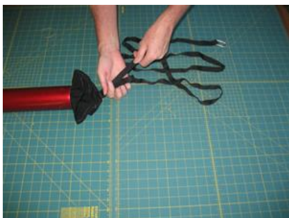
Step 10 - Z-Fold your shock cord. IMPORTANT: Do not coil up the lines. They can form a knot.
