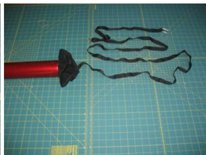
Step 9 - Now you can pack your chute into the airframe. First put in your chute protector. I use a Fruity Chute Nomex protector for this.
