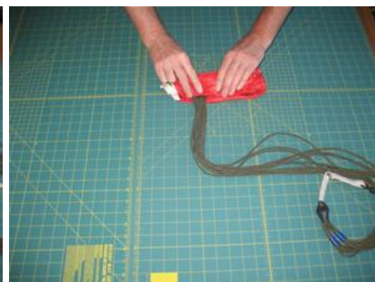
Step 8 - Now start to wrap the shroud lines around the chute. Note that the back of the chute is smooth with the material all pulled around into the crease.
