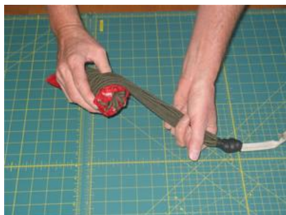
Step 8 (cont) - Stop when you reach the end of the chute. IMPORTANT: Note that the shroude lines stop wrapping and exit on the same end as the lines connect to the canopy. Again this assures that they can't wrap over the end of the chute.
