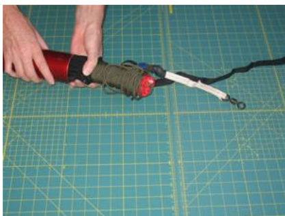
Step 13 - Now push in the chute with the shoud lines going in last. Make sure the protector folds around the chute evenly so protection is maximized around the entire chute.
