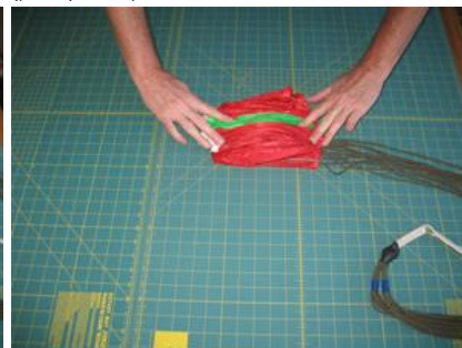
Step 5 - Pull the fabric on the underside of the chute around the edge and onto the top. You want the fabric on the underside smooth with no folds.
