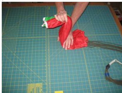
Step 4 - "Z" fold the chute into thirds.
