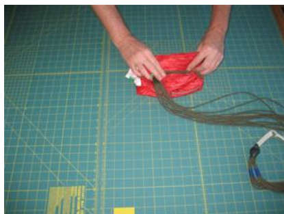
Step 7 - Bring the shroud line bundle up the crease to about 1/3 or the distance from the end. IMPORTANT - Do not bring the shroud lines to the very end. It is important that you do not allow a shroud line to wrap over the end of the chute and possibly result in a tangle!
