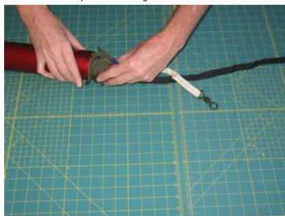
Step 13 (cont) - Be sure the last wrap of shroud lines goes in cleanly. If you have to force the chute in you probably have a problem.
