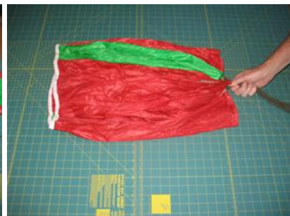
Step 2 - Grab all the shroud lines and organize the gores (panels) of the parachute.
