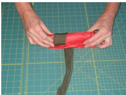
Step 8 (cont) - As I wrap note how the lines are not twisted. IMPORTANT: Don't just grab the lines and wrap these like you might wind kite string on a spool. Each wrap will result in a twist!
