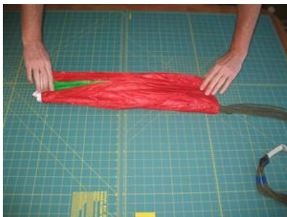
Step 3 - Fold over the gores on both sides towards the center. You want to organize the chute until it is about 15% of the diameter of the chute size. For a 42" chute it should be about 5" wide.
