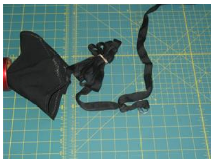
Step 11 - Once you have Z-folded the shock cord wrap a little rubber band around it - loosely so it comes off easily. It's there to keep the cord organized.
