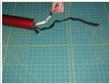
Step 14 - Now quick-link the chute to your rigging and nose cone. Pop on your nose cone and your DONE!
